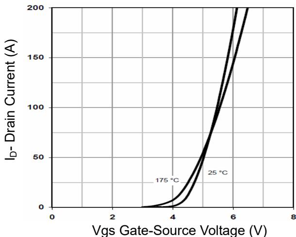
**Figure 2 Transfer Characteristics**
