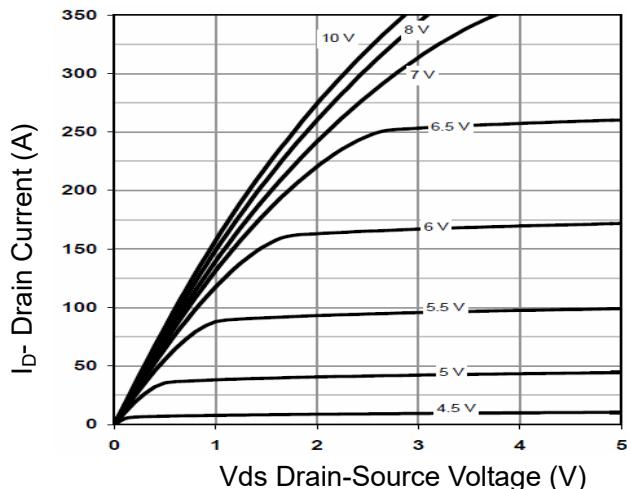
**Figure 1 Output Characteristics**
